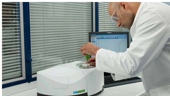
FT-IR Polymer ID Analyzer - Spectrum Two instrument
