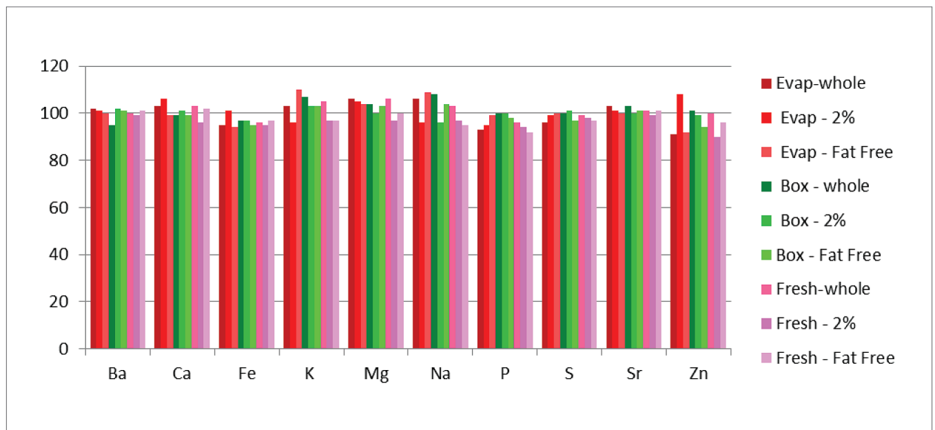
Figure 3. Spike recoveries in milk samples (evaporated milks in shades of red; boxed milks in shades of green; fresh milks in shades of pink).
